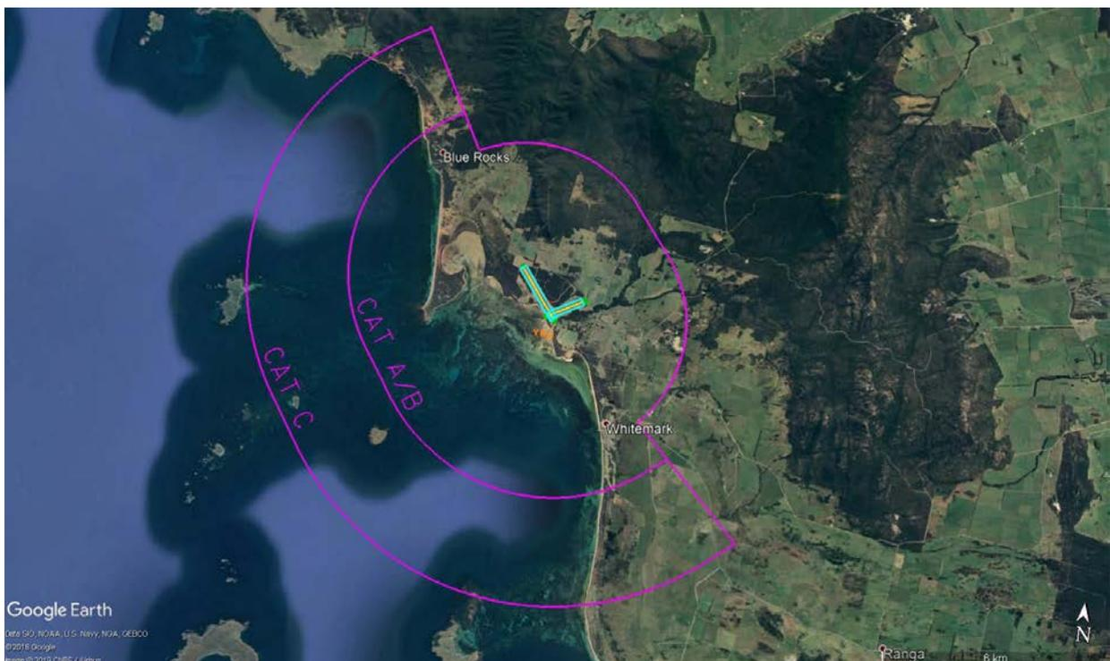
**Figure 3: Circling areas for aircraft (Cat C area only to be lowered)**
