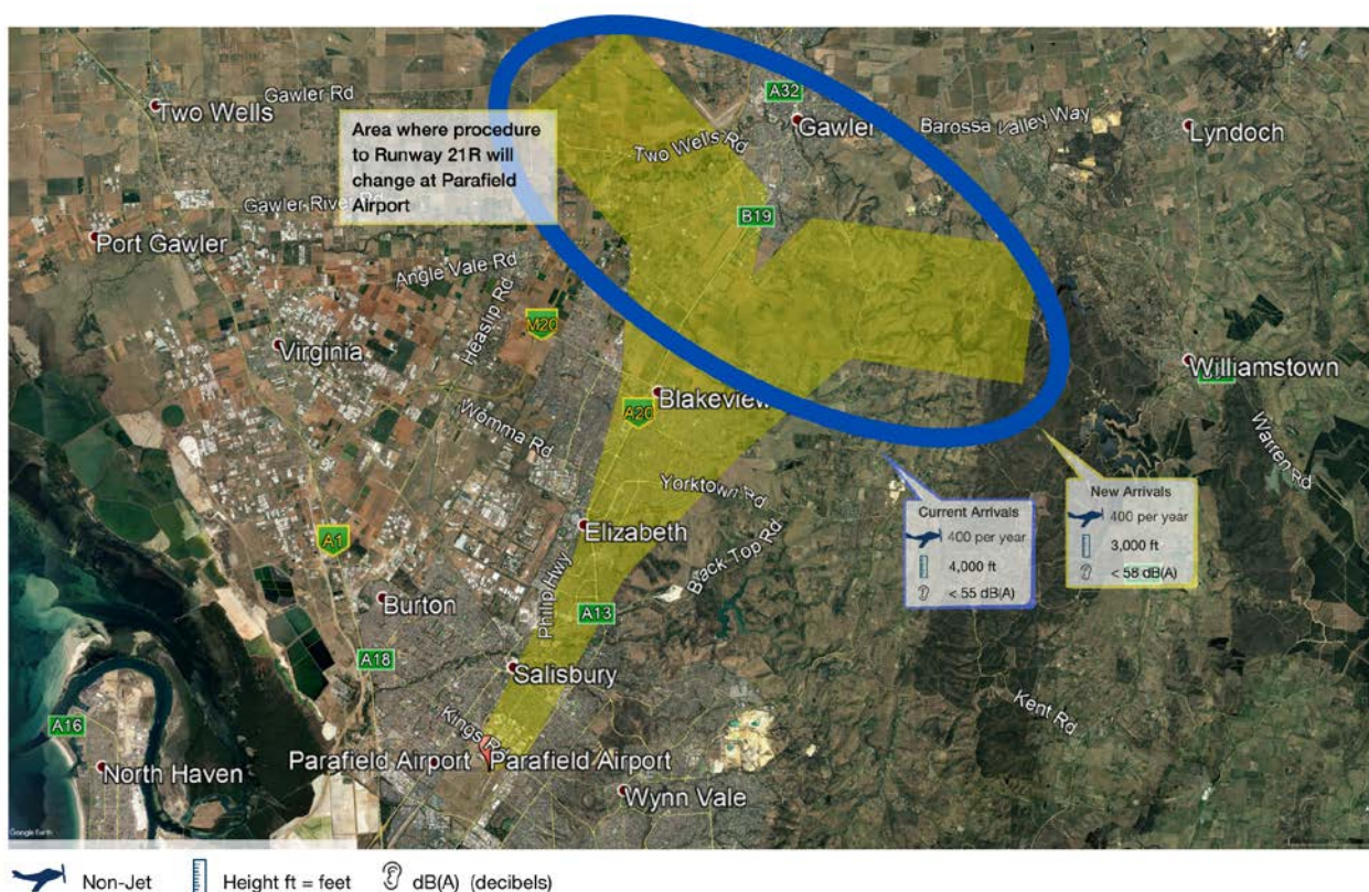
Figure 1: Approach to Runway 21R existing and changed approach procedures (yellow) with no lateral change, area where aircraft may operate at lower heights (blue circle).
