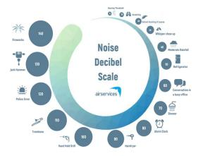
**Figure 9**: Noise Decibel Scale (Source: Noise Navigator® Sound Level Database) provides examples of the level of noise (decibels) that various activities and equipment emit, and communities may experience. The diagram is not designed to illustrate the entire effect of aircraft operations.
